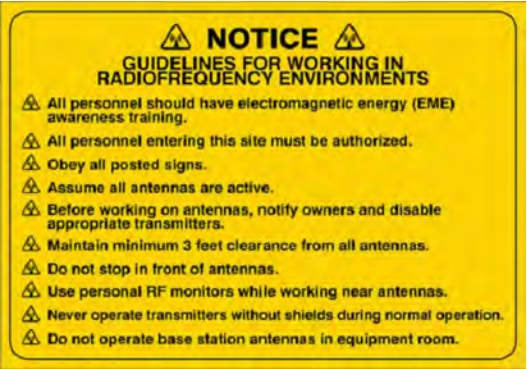
② RF GUIDELINES SIZE: 6”X 4” (TO BE MOUNTED ON GATE)
