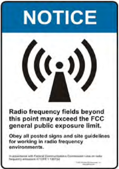
③ RF WARNING SIGN SIZE: 10”X 14” (TO BE MOUNTED ON GATE)
